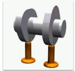
• The cam pictured here would be reversible, as it is symmetrical (the same on both sides, if cut in half).
